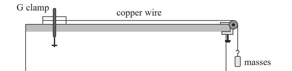
The work done in stretching the wire is given by the area under which graph?
