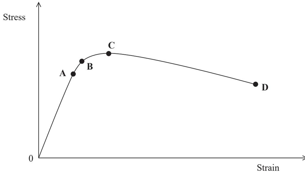
Which point would give the value for maximum tensile stress?
